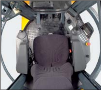
Operators compartment with driving controls integrated in the seat
