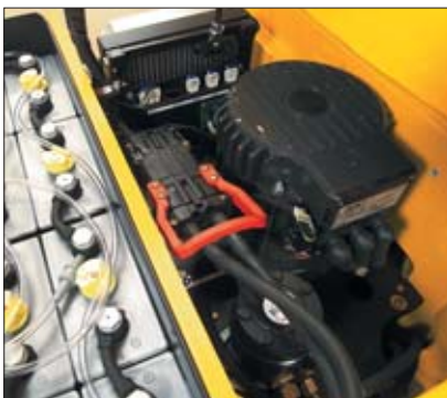
Drive and lift motor with AC technology
