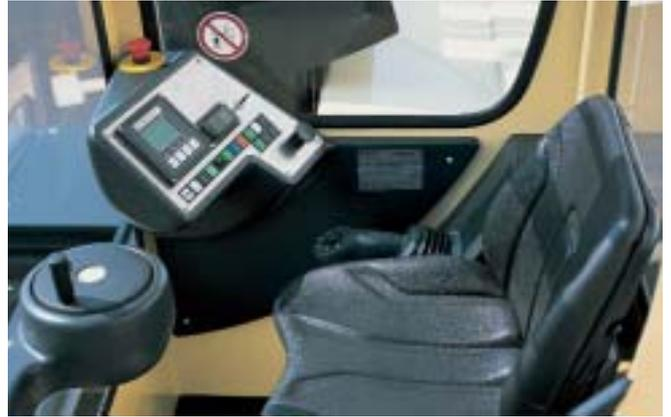
Drivers enjoy operating HUBTEX sideloaders. Everything is clearly arranged and easily accessible. Sensitive full power, multidirectional steering with fingertip control give HUBTEX trucks extreme manoeuvrability with millimetre accuracy allowing them to operate quickly and easily in the tightest corners. All hydraulic functions like the direction pre-select are operated via a modern joystick control, developed by HUBTEX.
