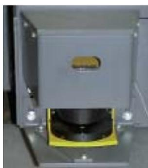
HUBTEX laser scanning system for the bystander safety when working in narrow aisles (option).
